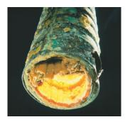
▲ FIGURE 18.22 Scale formation. The interior of this water pipe has been coated with CaCO<sub>3</sub> and other insoluble salts deposited from hard water.
