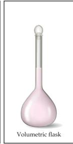
Volumetric flask **contains** a specific volume
