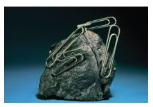
▲ FIGURE 23.6 A permanent magnet. Permanent magnets are made from ferromagnetic and ferrimagnetic materials.
