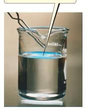
Seed crystal of sodium acetate added to supersaturated solution
