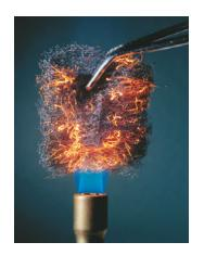
Steel wool heated in air (about 20% O<sub>2</sub>) glows red-hot but oxidizes to Fe<sub>2</sub>O<sub>3</sub> slowly
