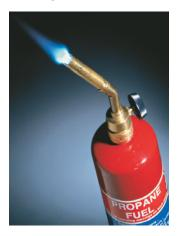
▲ FIGURE 3.8 Propane burning in air. Liquid propane in the tank,  $C_3H_8$ , vaporizes and mixes with air as it escapes through the nozzle. The combustion reaction of  $C_3H_8$  and  $O_2$  produces a blue flame.
