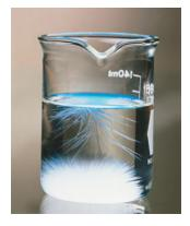
Excess sodium acetate crystallizes from solution
