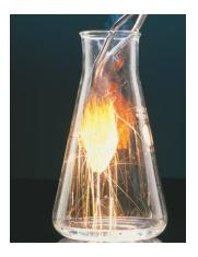
Red-hot steel wool in 100% O<sub>2</sub> burns vigorously, forming Fe<sub>2</sub>O<sub>3</sub> quickly
