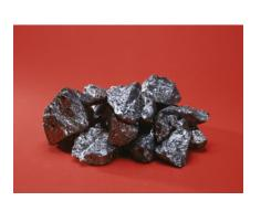
▲ FIGURE 7.18 Elemental silicon. Although it looks metallic, silicon, a metalloid, is brittle and a poor thermal and electrical conductor.
