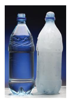
▲ FIGURE 11.12 Expansion of water upon freezing.
