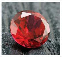
▲ FIGURE 12.25 Brittleness and faceting in ionic crystals. (a) When a shear stress is applied to an ionic solid, the crystal separates along a plane of atoms as shown here. (b) This property of ionic crystals is used to facet gemstones, such as rubies.
