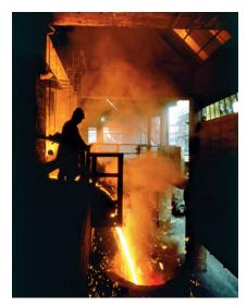
▲ FIGURE 6.5 Color and temperature. The color and intensity of the light emitted by a hot object, such as this pour of molten steel, depend on the temperature of the object.
