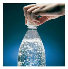
▲ FIGURE 13.16 Gas solubility decreases as pressure decreases. CO₂ bubbles out of solution when a carbonated beverage is opened because the CO₂ partial pressure above the solution is reduced.
