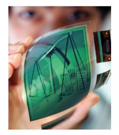
▲ FIGURE 11.35 Electronic paper (e-paper) based on cholesteric liquid crystal technology.
