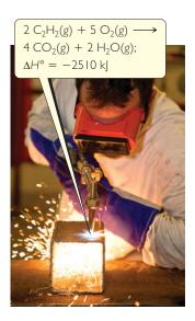
▲ FIGURE 22.13 Welding with an oxyacetylene torch.
