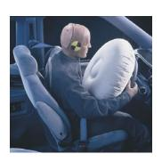
▲ FIGURE 3.7 Decomposition of sodium azide, NaN<sub>3</sub>(s), is used to inflate automobile air bags.
