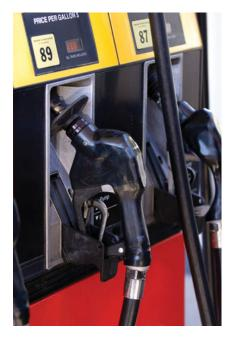
▲ FIGURE 24.6 Octane rating. The octane rating of gasoline measures its resistance to knocking when burned in an engine. The octane rating of the gasoline in the foreground is 89.
