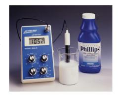
▲ FIGURE 16.6 A digital pH meter. The device is a millivoltmeter, and the electrodes immersed in a solution produce a voltage that depends on the pH of the solution.
