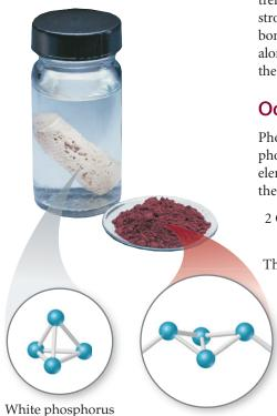
▲ FIGURE 22.27 White and red phosphorus. Despite the fact that both contain nothing but phosphorus atoms, these two forms of phosphorus differ greatly in reactivity. The white allotrope, which reacts violently with oxygen, must be stored under water so that it is not exposed to air. The much less reactive red form does not need to be stored this way.
